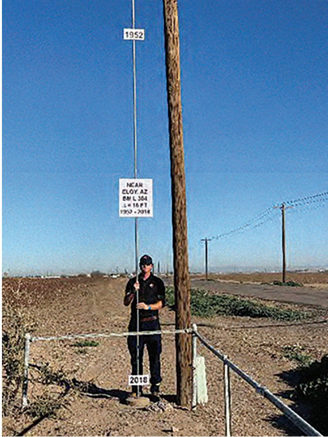
Land subsidence Eloy-Picacho, Pinal County. Signs on the pole show approximate altitude of land surface in 1952 and 2018. Source: ADWR.
